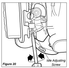
The engine must return to idle speed whenever the throttle lever is released. Idle speed is adjustable, and must be set low enough to permit the engine clutch to disengage the cutting attachment.
